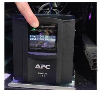
6. All components should power down immediately. The device is fully powered off when the display screen on the UPS goes dark.
