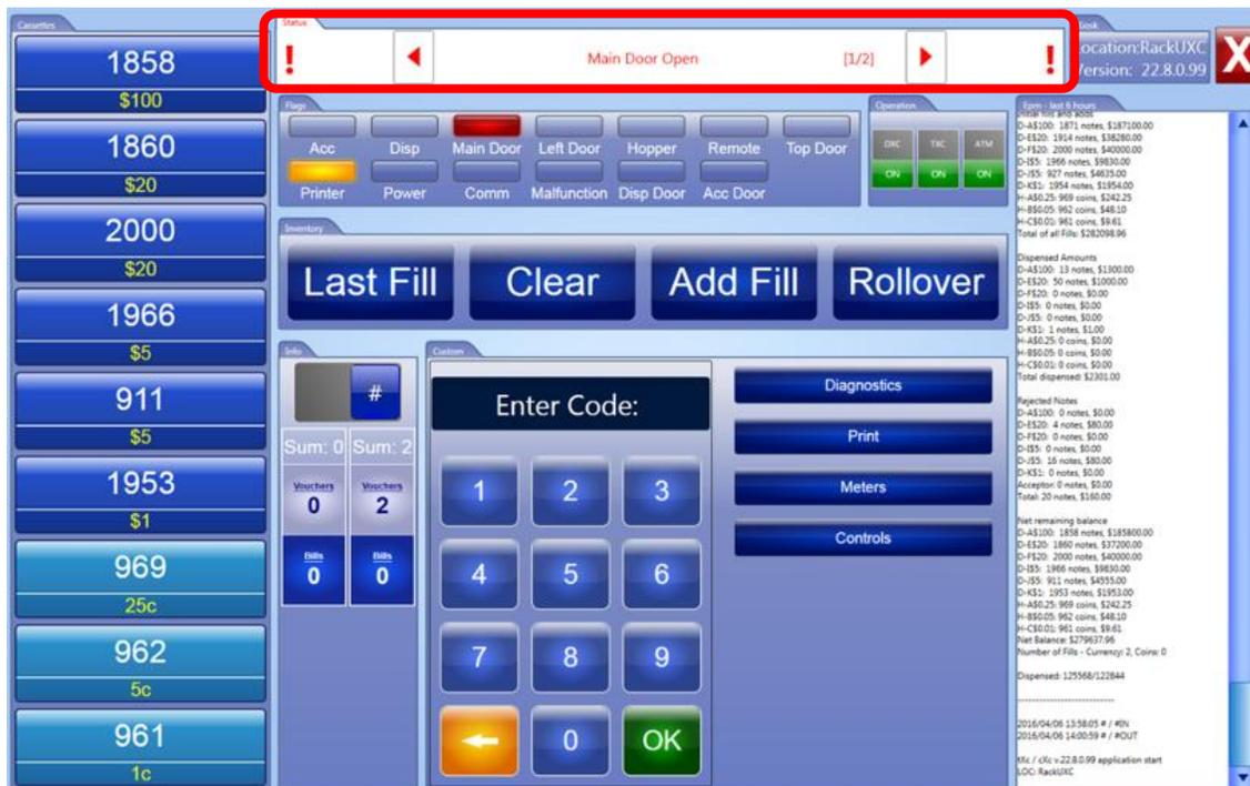
3. Perform a visual inspection and correct the error as needed. If the error is not apparent, the attendant can further diagnose the nature of the problem as follows:
