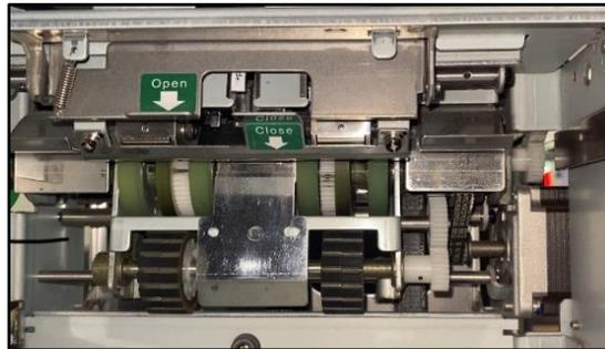
**Note:** At the back of the dispenser pockets are two metal tabs labeled with green arrows that both point down, one is labeled **Open** and the other is labeled **Close**. Reach into dispenser pocket and push down on the metal tab with green arrow labeled **Close**. When pushing down, you should hear a click, this indicates that the Pick Module is in its correct closed position. This is a common issue that causes many rejects and is easily corrected by pushing down on the metal tab.
